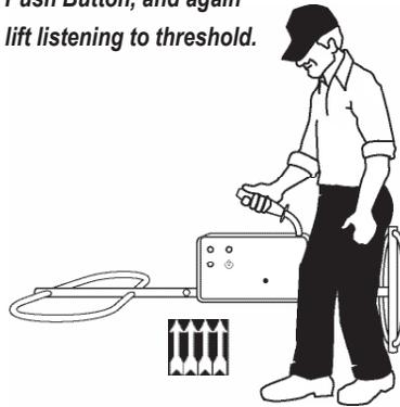
*Lift about six inches if threshold increases, turn Ground Balance slightly clockwise, (+) lower, press & release Push Button, and again lift listening to threshold.*
