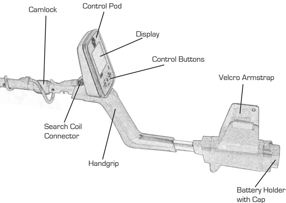
7. Grip the detector and sweep the search coil over the floor. If the fit feels uncomfortable, adjust the position of the lower fiber rod. The ideal position allows you to stand up straight and sweep the search coil over the ground without stooping over.
